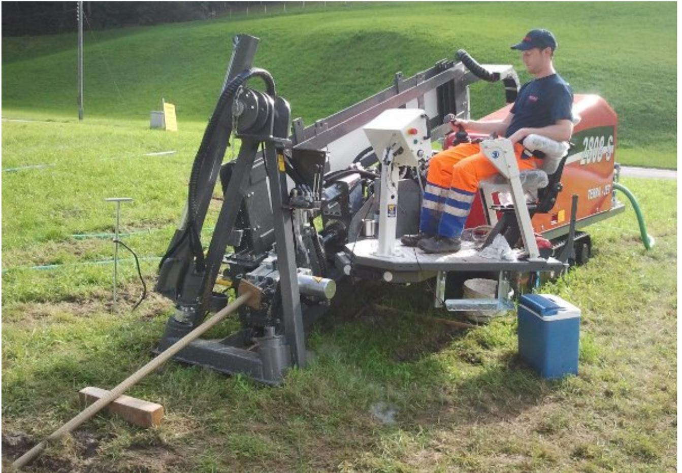
In the little Swiss city Mümliswil the TERRA-JET 2808 S laid a pipe bundle consisting of three pipes underneath the „Mümliswiler Bach“ (small river in Mümliswil). This pipe bundle consisted of a protection pipe OD 132 mm (5.2“) for electricity, a protection pipe OD 92 mm (3.6“) for fibre optic and a pressure pipe OD 63 mm (2.5“) for water. The pilot bore had to be reamed in steps up to ø 360 mm (14“). Then the pipe bundle could be pulled in.
