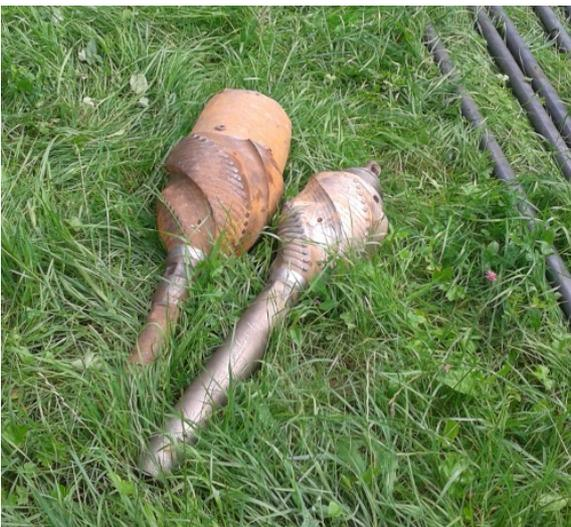
The 49 m (162 ft) long pilot bore was reamed with these two backreamers up to  $\varnothing$  215 mm (8.5") and then finally to  $\varnothing$  360 mm (14").
