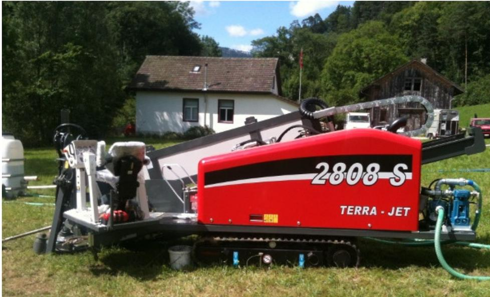
The rack and pinion drive has proved its value also at this jobsite. It provides thrust and backream forces of 80 kN (8 tons, 17'600 lbs). →
