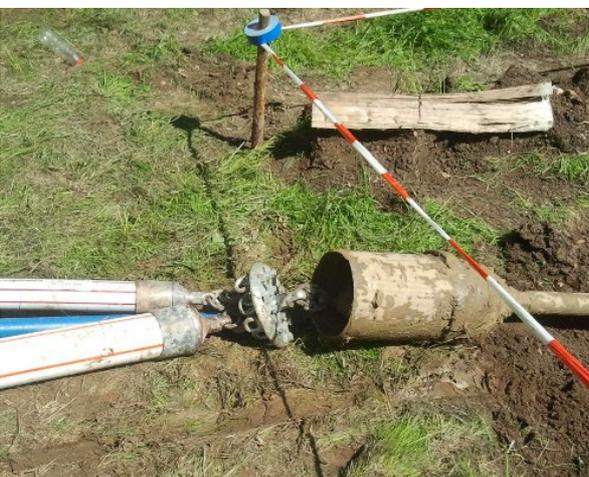
The backreamer  $\varnothing$  360 mm (14") with pipe bundle (1x OD 132 mm, 1x OD 92 mm, 1x DA 63mm)
