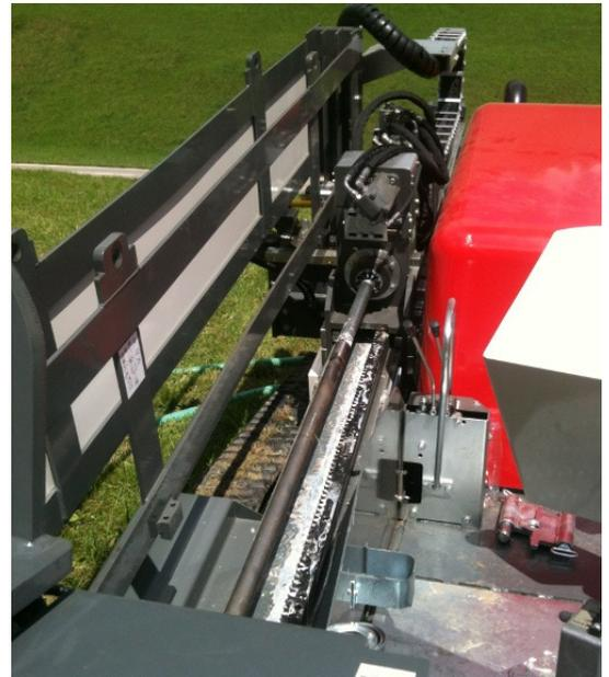
The backreamer  $\varnothing$  360 mm (14") has pulled in the pipe bundle over 49 m (162 ft) successfully. ↓
