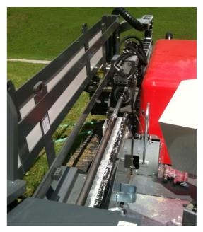
The backreamer ø 360 mm (14") has pulled in the pipe bundle over 49 m (162 ft) successfully.
