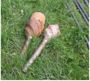
The 49 m (162 ft) long pilot bore was reamed with these two backreamers up to  $\emptyset$  215 mm (8.5") and then finally to  $\emptyset$  360 mm (14").
