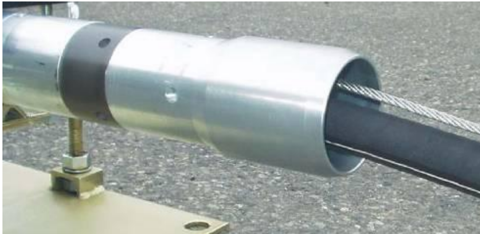
The TERRA-HAMMER TU 068/75plus SK with the end sleeve \varnothing 75 mm (2.95"). This end sleeve \varnothing 75 mm (2.95") allows to pull in HDPE pipes OD 63 mm (2.5").
