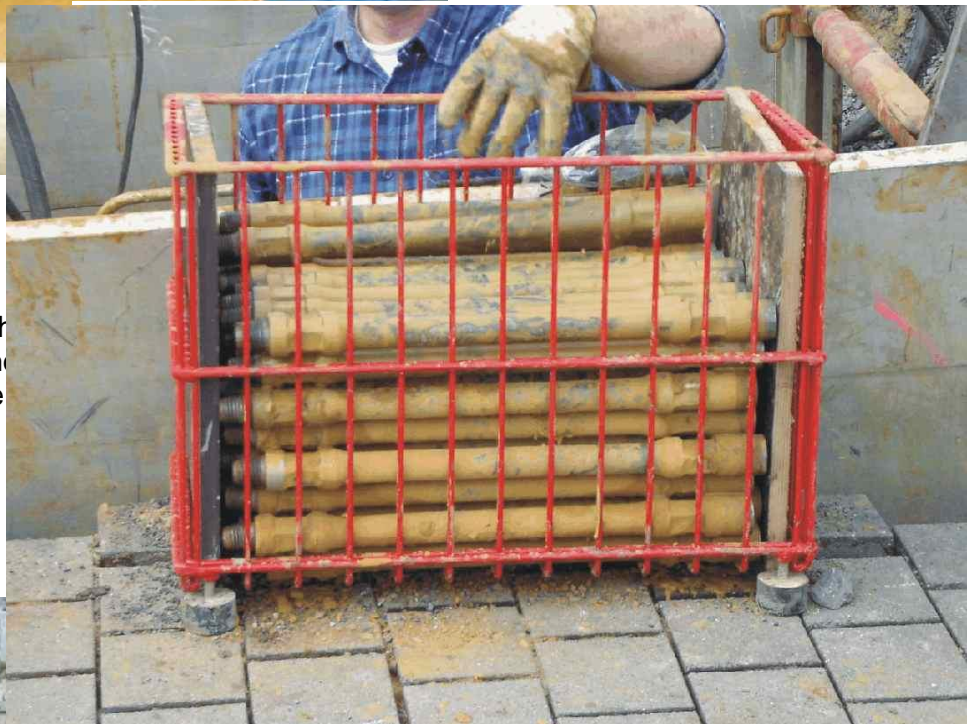
Pic. right: M/s Gerhard Rode has built their own rod boxes. They allow the cleaning of the drill rods either outside or inside.
