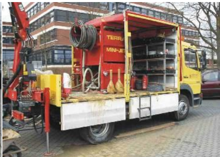
This truck with rear crane was purchased by M/s Gerhard Rode especially for the TERRA MINI-JET.
