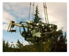
The TERRA-DRILL TD 150x7 V was lifted into the drilling area by a truck crane. Then the drill rig could drive with its rubber crawler around the houses into the drilling position.
