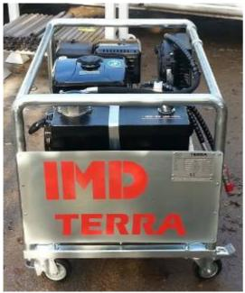
The hydraulic power pack and the rods are prepared. The power pack has an electric starter and an optional oil cooler.
