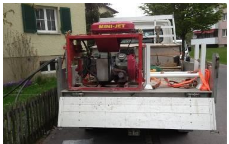
A hydraulic power pack drives the TERRA-JACK 125.
