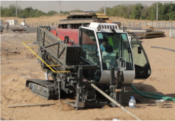
The TERRA-JET 8522 S during the drilling operation. The comfortable driver's cabin is equipped with a powerful air conditioning (cooling capacity over 6 kW).
