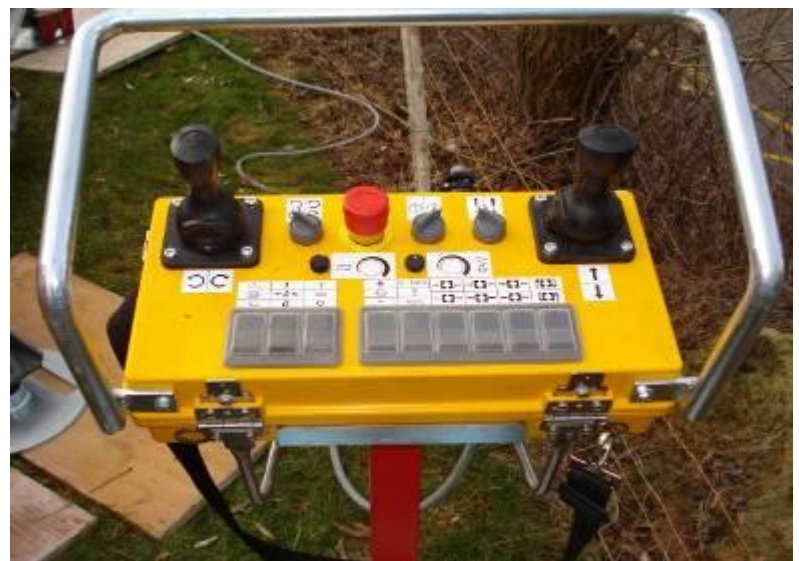
This remote control controls the complete drill. The left picture shows the triplex clamping and breaking system. The two upper clamps swing sidwise hydraulically.
