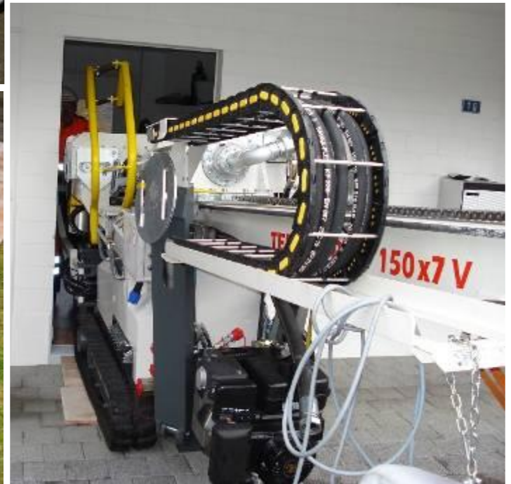
The TERRA-DRILL 150x7 V is only 0.95 m (3.14 ft) wide in its transportation mode. So it can drive through 1.0 m (3.3 ft) wide doors.
