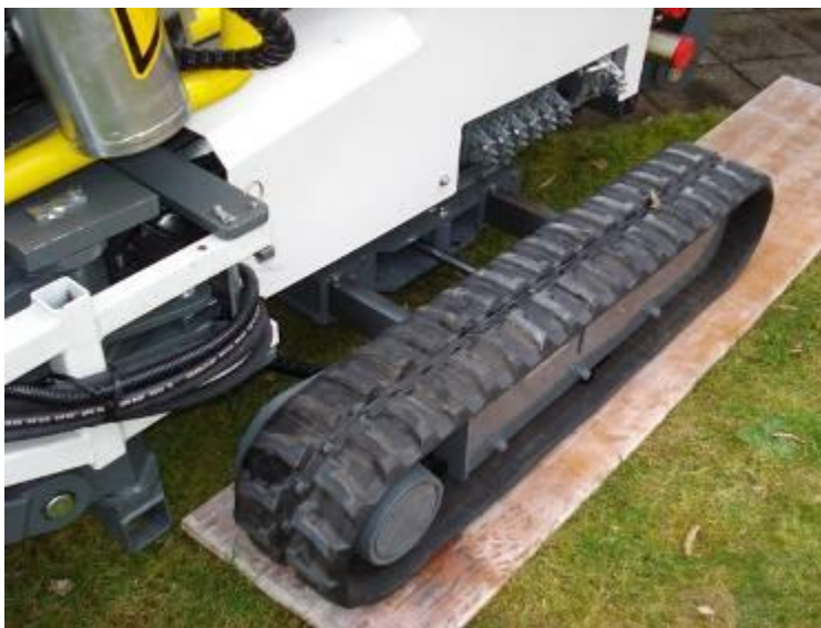
The rubber crawler can be adjusted hydraulically in its width (telescopic crawler).
