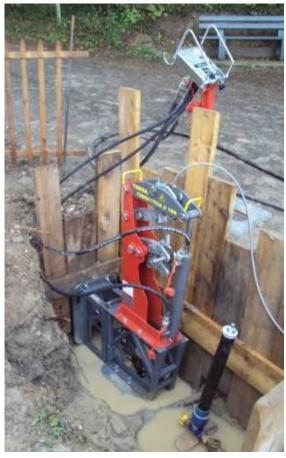
The TERRA-EXTRACTOR X 100 in the pit. The operation is done with the control station on top of the pit.
